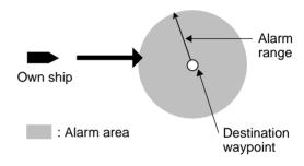
Figure 9-3 How the arrival alarm works
